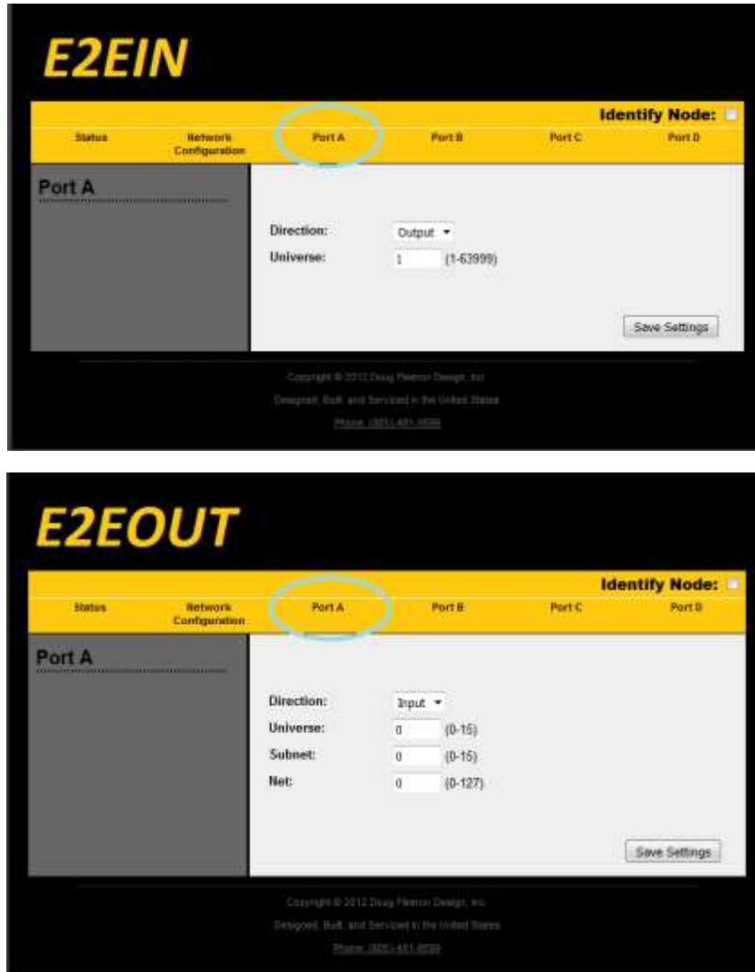
Figure 2: An E2E's virtual Port A configuration for sACN in and ArtNet out
